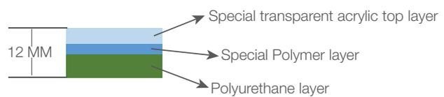
**Special transparent acrylic top layer** has a high chemical resistance to: cleaning agents, perfumed foams, household detergents, body care products. It prevents surface defects, crazing/cracking, decoloration and color fading
