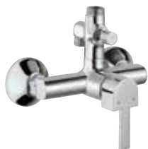
DRC-37145 Single Lever Exposed Shower Mixer With Provision For Connection to Exposed Shower Pipe (SHA-1211NH & SHA-1213) & Hand Shower With Connecting Legs & Wall Flanges Rs. 5,400
